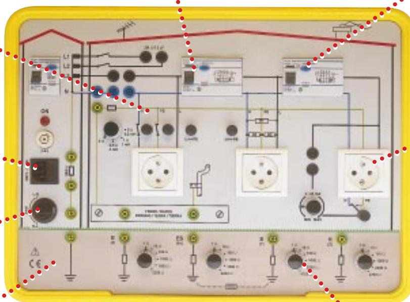
The different possible earth connections enable simulations on earth-to-earth, earth-to-neutral and insulated to earth networks. Parallel earth connections are also possible.
